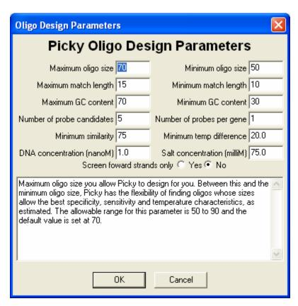
Picky allows the parameters to be specified for oligo size, match length, sensitivity, GC content and melting temperature difference. The following is a description of each set of parameters:
